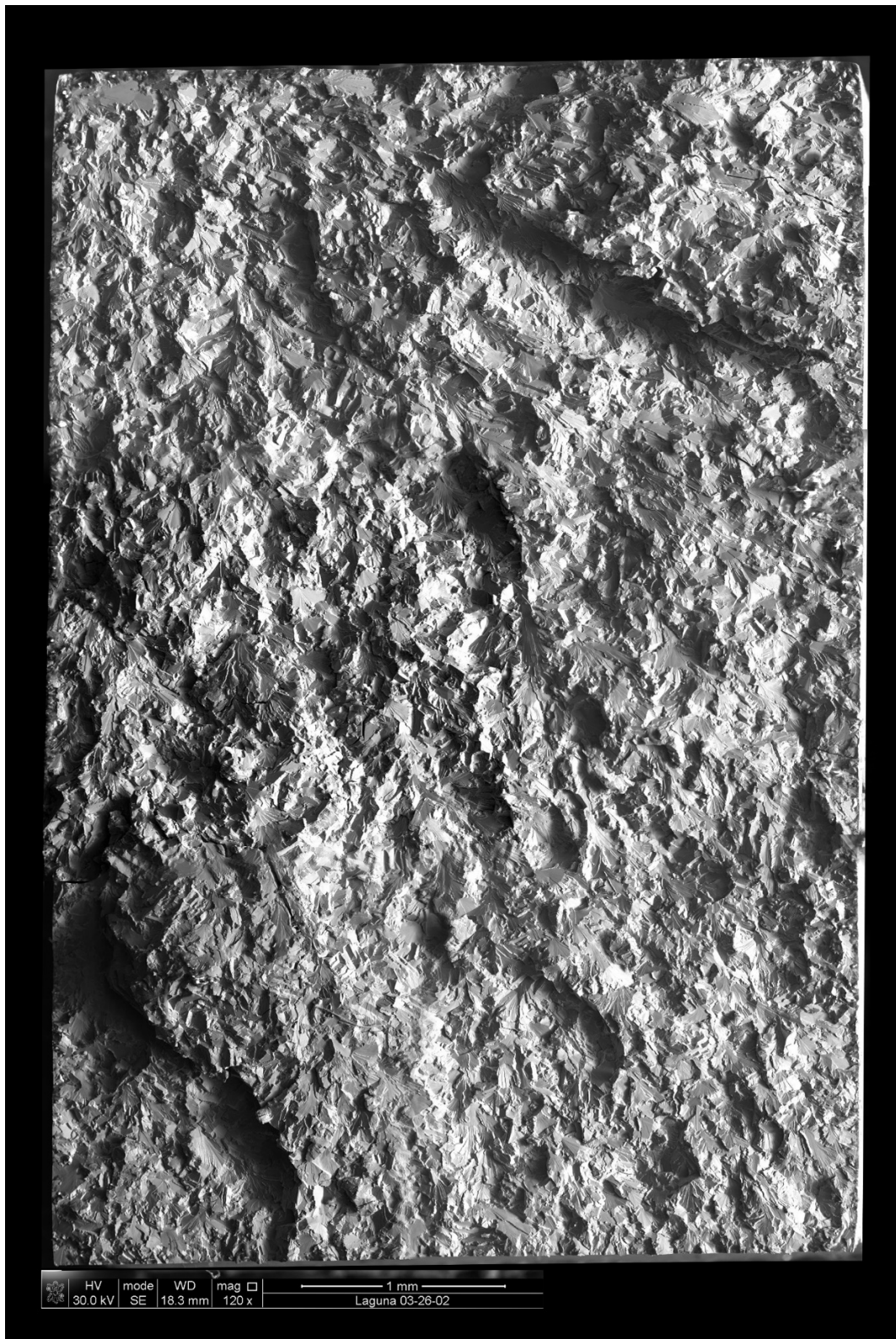
Fig. 16. SEM of the whole fracture surface (lighter contrast)
