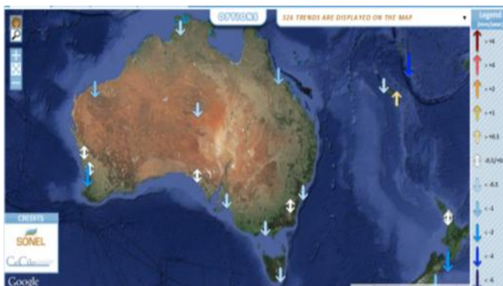
Fig. 13. Absolute vertical velocities of GPS domes in Australia computed by SONEL (image from [36])
