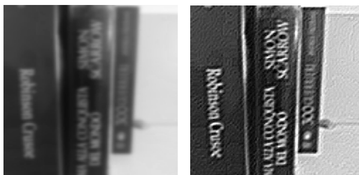
Figure 15. Result of deblurring on a comprehensive image set (Image 11_IM): (Left) input image; and (Right) output of the ICA neural system.
