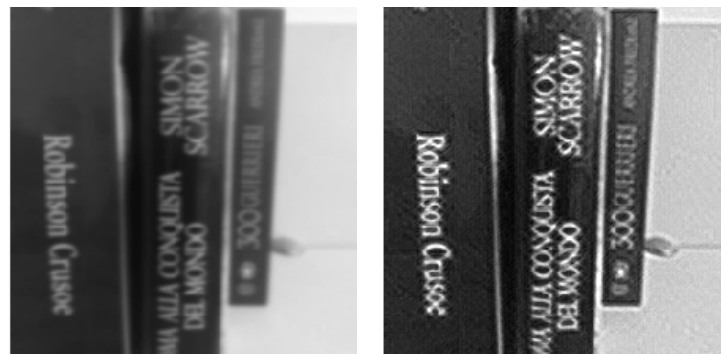
Figure 14. Result of deblurring on a comprehensive image set (Image 12_IM): (Left) input image; and (Right) output of the ICA neural system.
