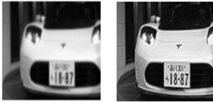
Figure 13. Result of deblurring on a comprehensive image set, in particular, on image 33_IM: (Left) input image; and (Right) output of the ICA neural system.
