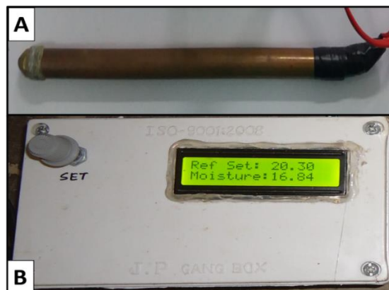
Fig. 1(A). Developed soil moisture sensor (sensing unit) (B) Controller and display units
