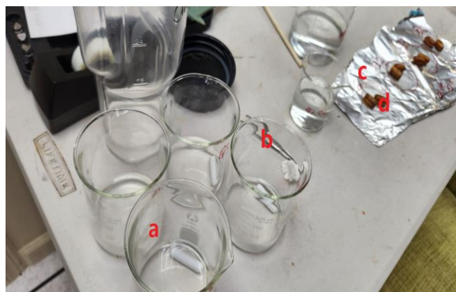
Fig. 3. Shows the beakers with sodium alginate (a) and calcium compounds with RO water. A forceps is found in (b), and the coated tablets (d) were placed on an aluminum foil (c)
