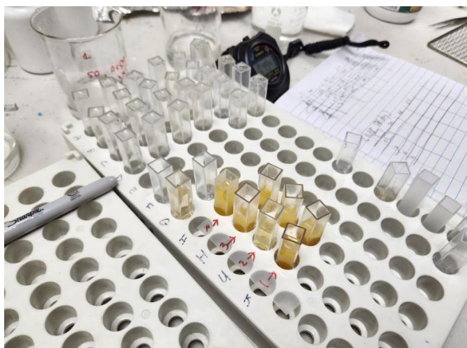
Fig. 5. Presents the aligned photometer cuvettes during our dissolution test. The samples were obtained every 20 minutes for up to 2 hours
