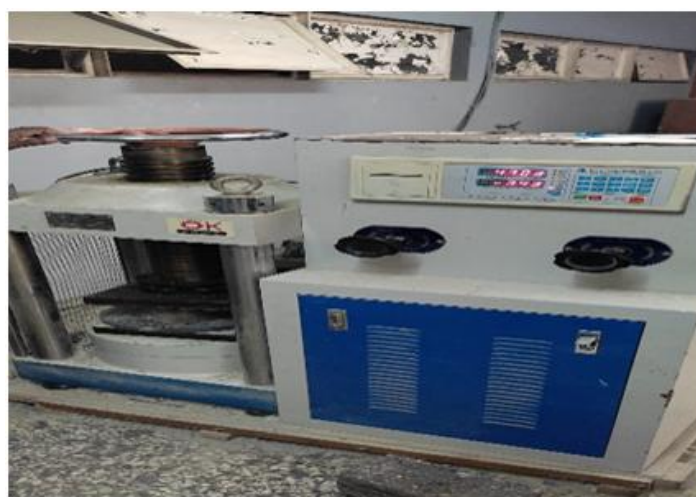
Fig. 4. Crushing of specimens
