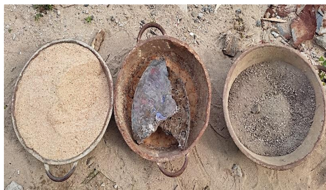
Fig. 2. Component materials: From left to right: sand, melted waste plastics, and granite
