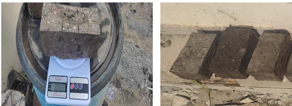
Fig. 3. Interlocking paving stone made from waste plastics
