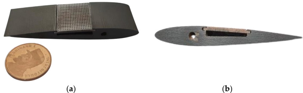
Figure 3. Model 3—Water jet cut model with Al perforated plate. (a) Isometric view; (b) sideview.
