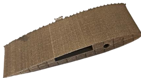
Figure 2. Model 2—metal 3D-printed airfoil.
