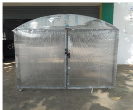
Fig. 4. Fabricated polycarbonate chamber
