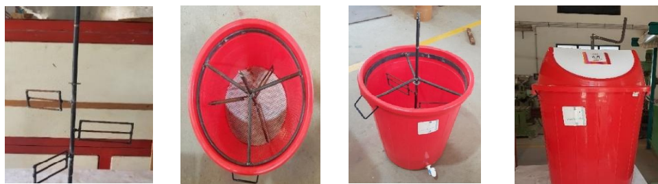
Fig. 6. Different views of the fabricated bio-digester
