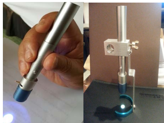
Fig. 1. A CXL-pen (made by New Vision Inc.) with battery-powered and adjustable spot size, operated by either hand-held (left) or a stand (right)
