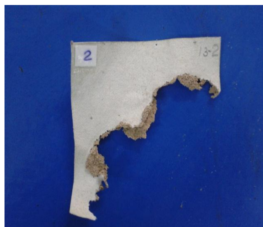
Fig. 5. Control sample eaten by termite
