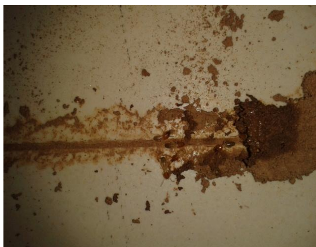
Fig. 4. Termite building termitorium on control sample
