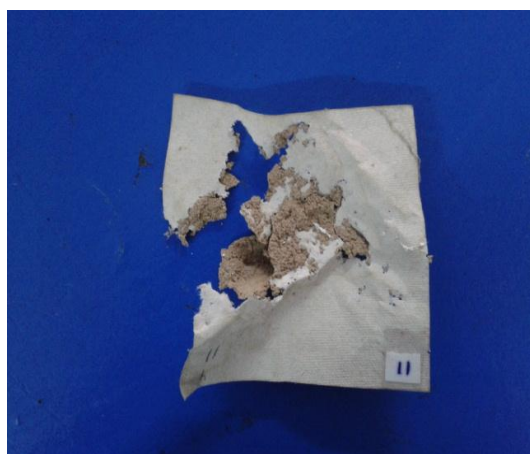
Fig. 5. Control sample eaten by termite
