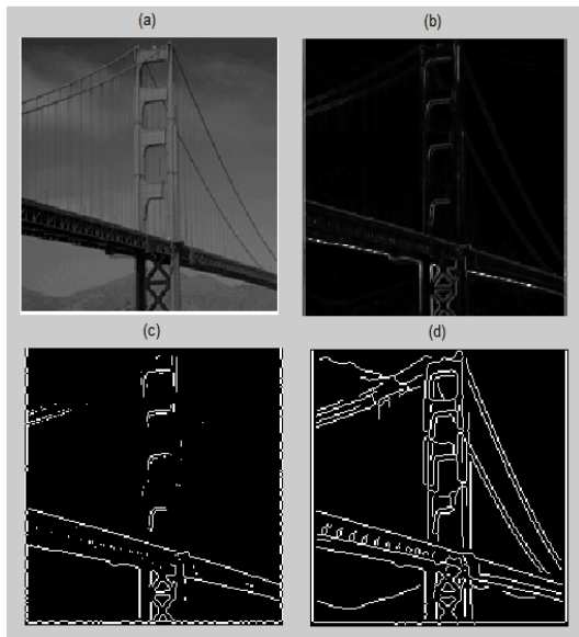
Fig. 18. Bridge image, (a) The original image, (b) Proposed technique result, (c) Sobel with threshold = 0.08, (d) Canny with proper threshold chosen by MATLAB
