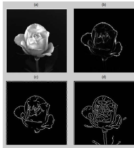
Fig. 19. Rose image, (a) The original image, (b) Proposed technique result, (c) Sobel with threshold = 0.08, (d) Canny with proper threshold chosen by MATLAB
