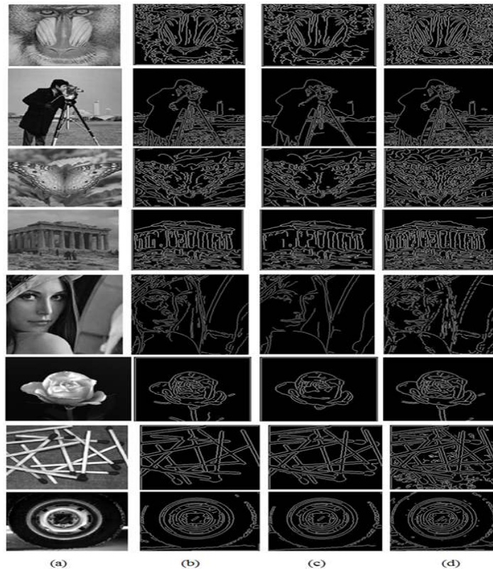
Fig. 22. Detailed images canny results (a) The original image, (b) Canny with proper threshold chosen by MATLAB, (c) Canny with threshold = 0.2, (d) Canny with threshold = 0.08
