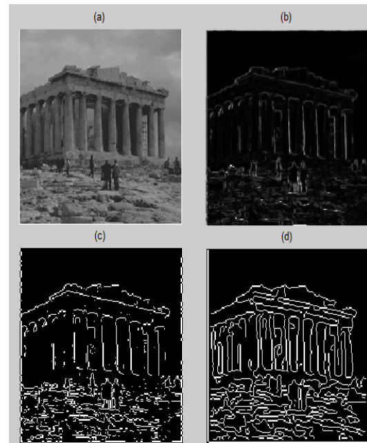
Fig. 15. Building image, (a) The original image, (b) Proposed technique result, (c) Sobel with threshold = 0.08, (d) Canny with proper threshold chosen by MATLAB
