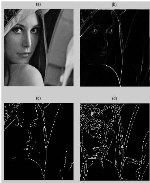
Fig. 16. Lina image, (a) The original image, (b) Proposed technique result, (c) Sobel with threshold = 0.08, (d) Canny with proper threshold chosen by MATLAB
