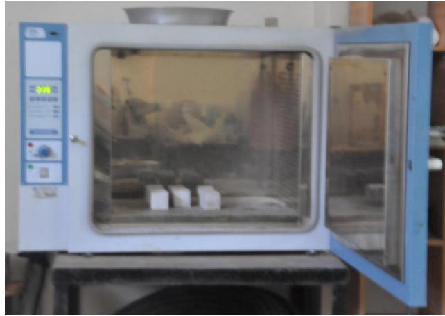
Fig. 2. Drying of specimens in an oven
