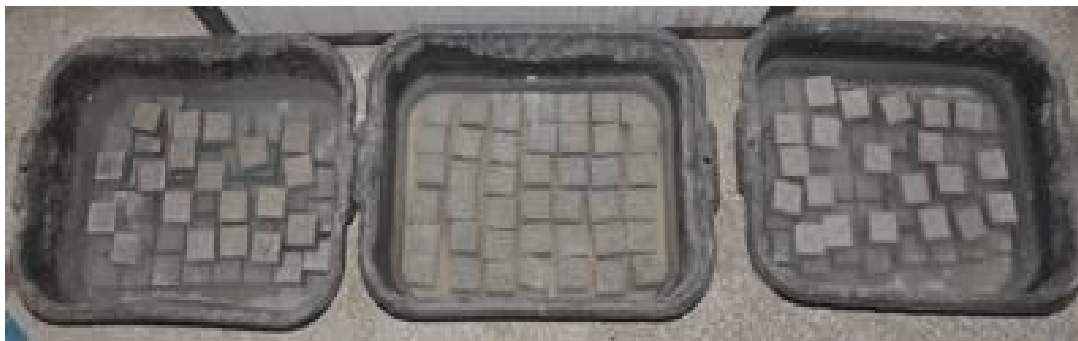
Fig. 1. Curing of specimens in water tanks
