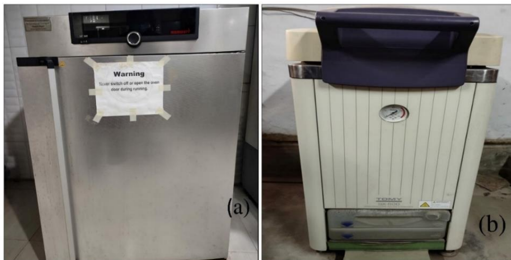
Fig. 2. Initial aspect to the design (a) Sterilize the Erlenmeyer flask by Microwave Oven for Spirulina cultivation (b) Zarrouk's medium was autoclaved by an Autoclave Machine
