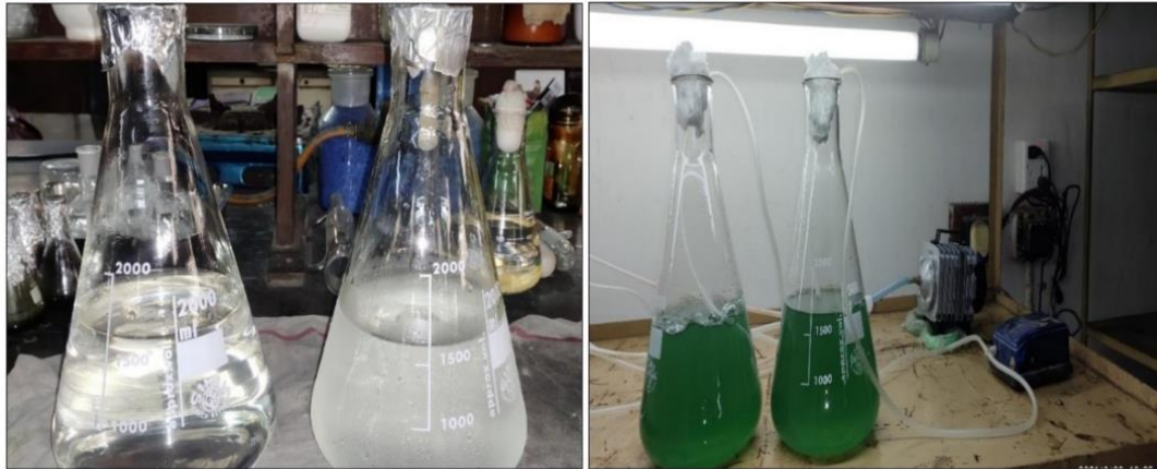
Fig. 1. (a): Zarrouk medium without \text{NaHCO}_3 (b) Extracting Supernatant added to the medium after autoclaving
