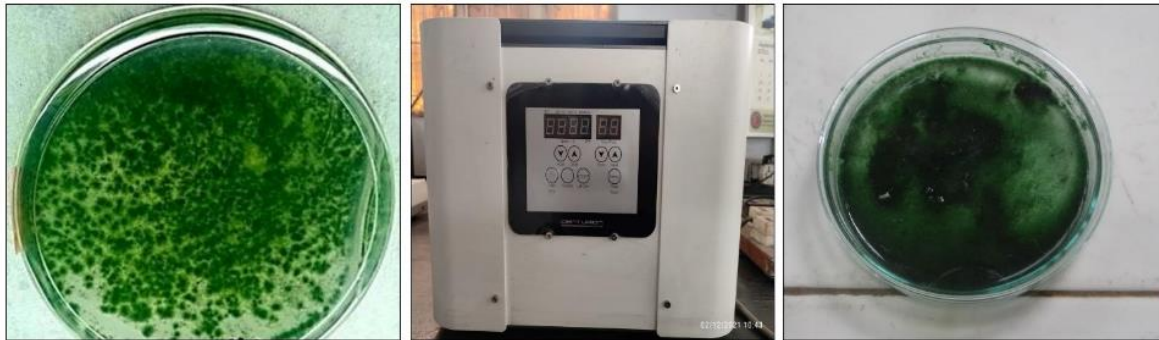
Fig. 4. Recovery of biomass by Centrifuge
