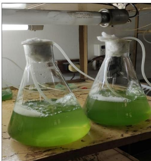
Fig. 3. CO 2 absorbent NaOH (left side) added to specific one flask and the other controls (right side)
