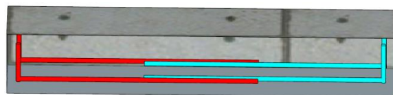
Fig. 5. 3D Schematic illustration of splice beam specimen for bond tests
