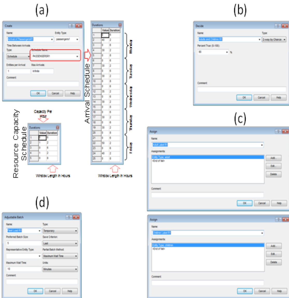
Fig. 4. Description of the Arena modules used for the simulation of the cab system (part I): (a) “Create” module for arrivals, (b) “Decide” module for separation of entities based on probabilities, (c) “Assign” modules for labelling of entities as “adult” and “children”, and (d) “Adjustable Batch” module for batch creation based on maximum size and waiting time
