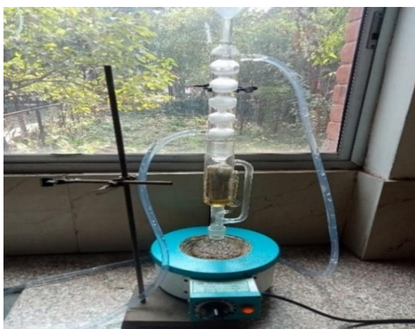
Image 6. Soxhlet extraction was used to extract the plant material
