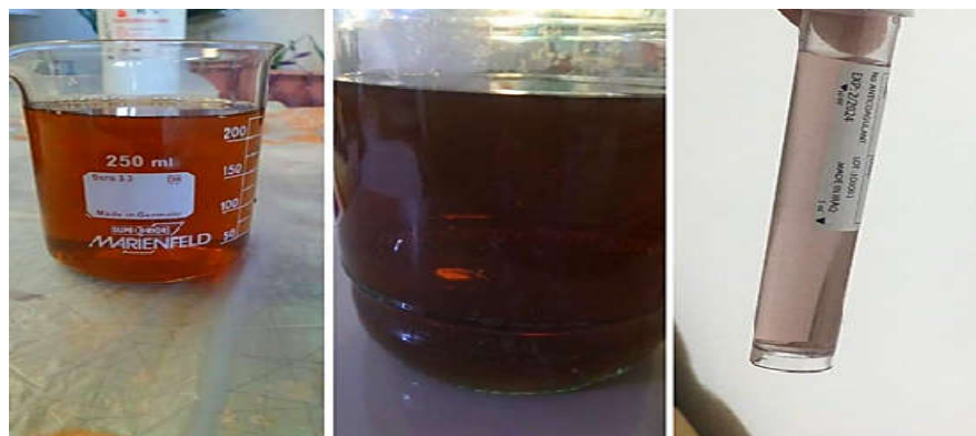
Fig. 5. The color change of the solution when forming silver AgNPs . particles
