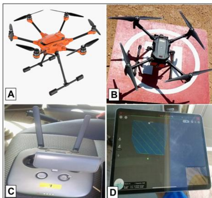
Fig. 6. (A) YUNEEC H250 Drone, (B) DJI Matrix 200 Drone, (C) Drone radio control, (D) Mission supervision tablet
