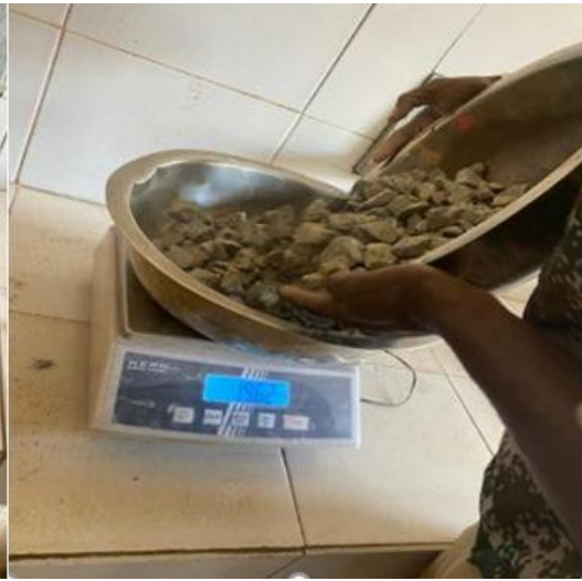
Fig. 3. Measurement of the mass of crushed aggregate
