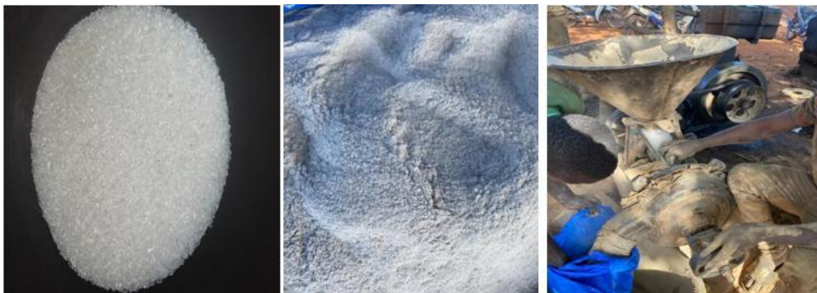
Fig. 1. Pictures showing glass grains and glass powder
