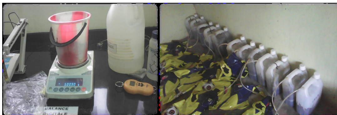
Fig. 3. The analytical balance (FX-2000i d = 0.01) and anaerobic reactors containing the feedstock at different SC
