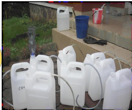
Fig. 2. Laboratory scale anaerobic digesters constructed from 5L plastic containers to assess the methanation process in situ
