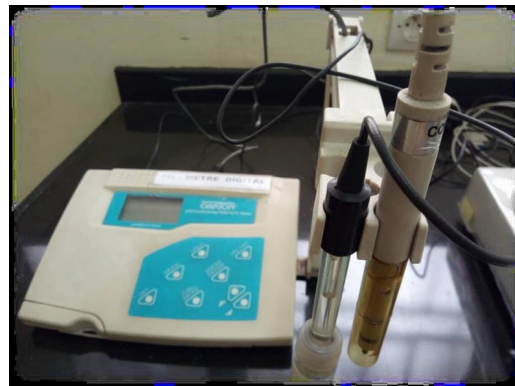
Fig. 7. Determination of pH using the OAKTON pH / CON 510 series pH meter
