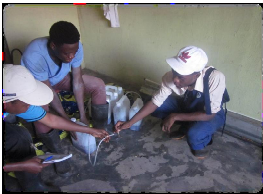
Fig. 5. Combustion test for qualitative evaluation of biogas
