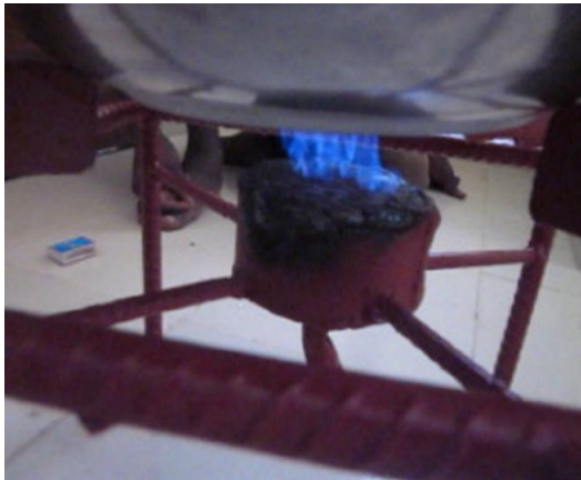
Fig. 4. A complete combustion of a biogas produced at GGC. The persistent blue flame confirm the presence of methane in significant proportion (50% or more)
